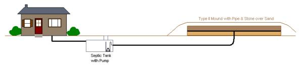
A type II mound is a private sewage system that consists of piping from the septic tank to the field. The effluent is pumped through a piping system that is above a bed of clean graded sand. The effluent then trickles through the sand bed to the natural soil surface. A type II mound is a reasonable option where there are shallow restrictive layers in the soil; a shallow water table or a below ground system cannot be located on the lot.
